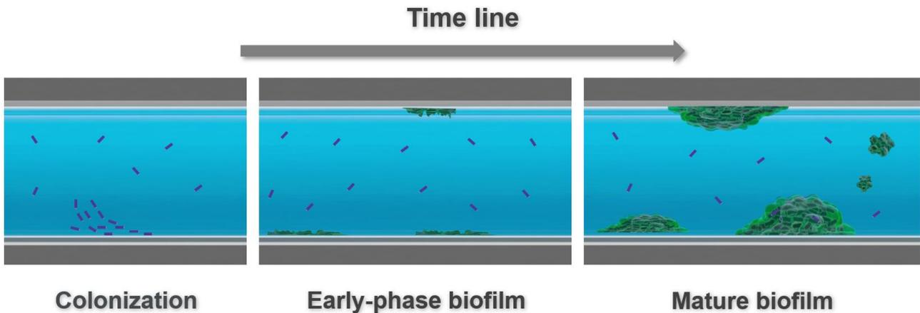
Figure 1: Development of biofilm, from the initial colonization of surfaces to its mature phase
